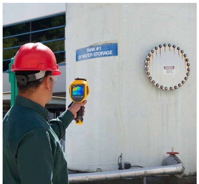
Thermal cameras can detect the level of fluid or other substance inside a tank, providing there is a temperature difference between the liquid, the air inside, and the air outside, and providing the tank is not made of a shiny material.
