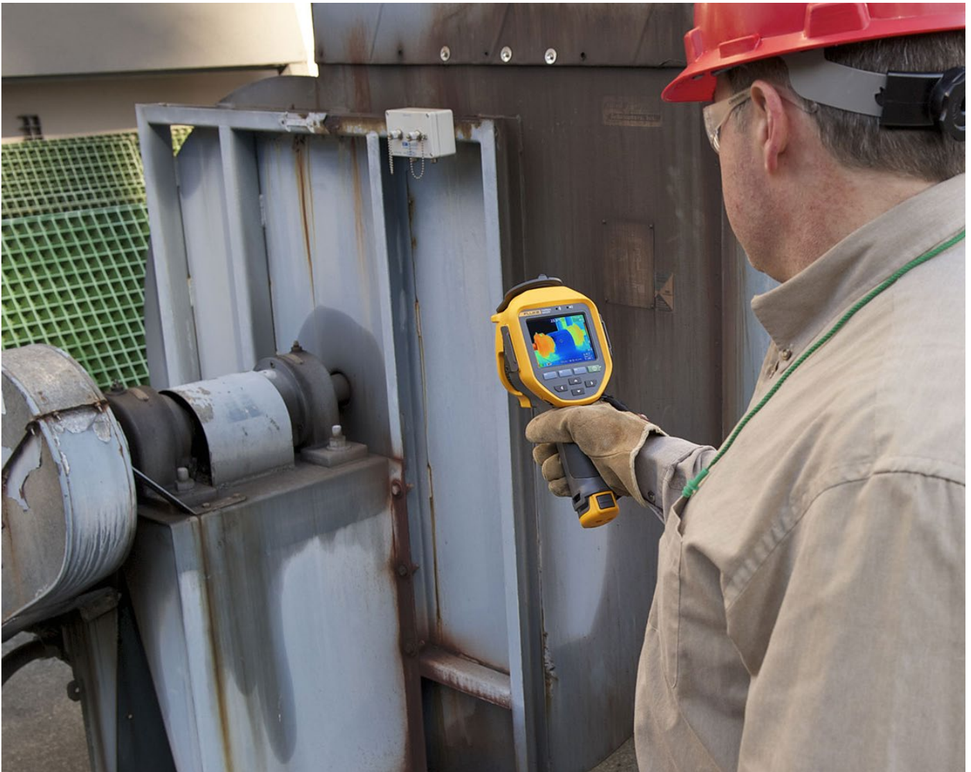
Shafts made of shiny stainless steel can be tricky to measure with thermal cameras. Compensate by measuring close to the coupling.
