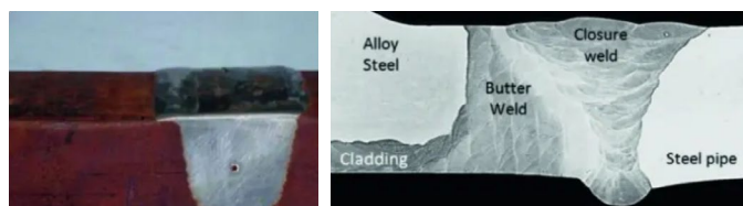
Figure 1: Common welds used in cladded pipes, including a dissimilar weld material (left) and a weld used to join two different materials (right).
