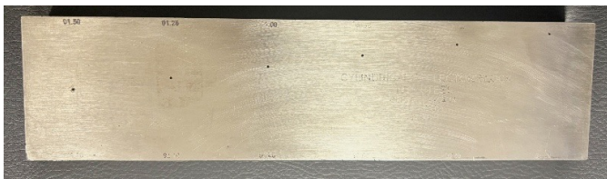
Figure 15: A Calibration Block for UT Inspections
