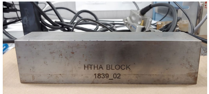
The second test configuration is a block with artificial HHTA with a 47mm thickness. Tests were conducted using a 10L64 A32 probe in contact mode.
