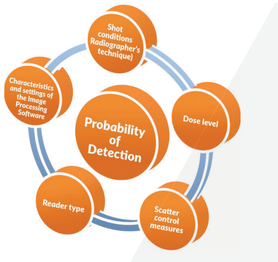
Figure 1: Factors that Influence the Probability of Detection in Radiographic Imaging Processes, based on White [7] [8].
