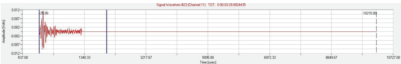
Figure 11 Short, sharp waveform typical of cracking.
